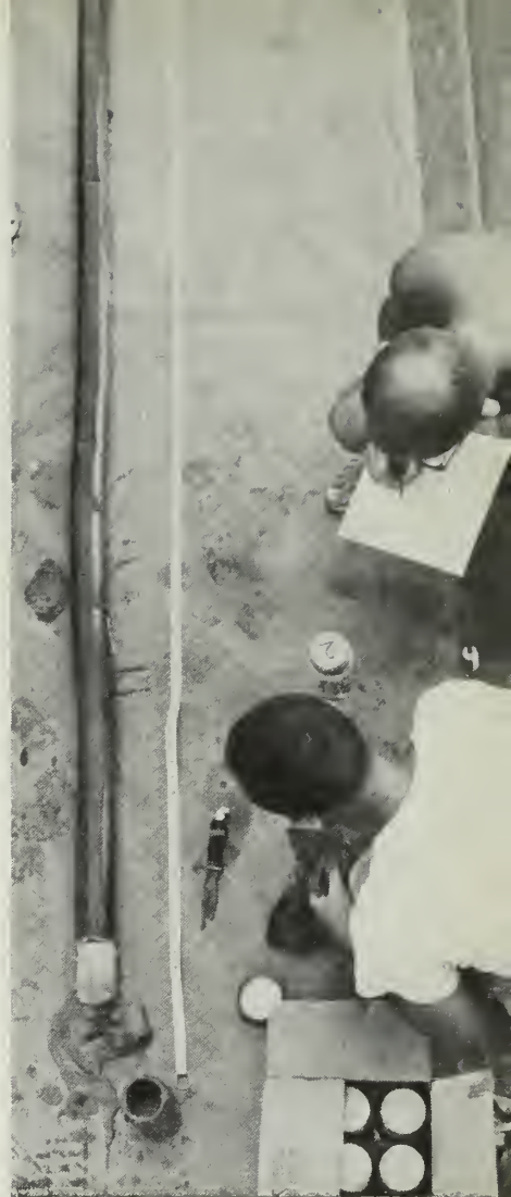
MUDDY MEASURE —Mud brought up by corer is checked. Below: Ewing corer is set for drop into ocean's floor.
